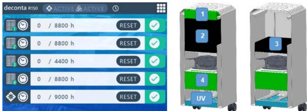
Abb. 14 Operating hours and recommended operating time of the individual stages
